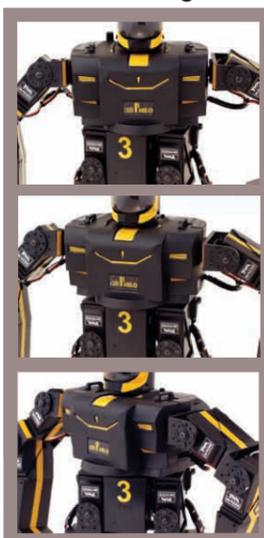
RoboPhilo comes with a powerful robot controller with 24 servo channels and up to 8 I/O interface. A specialized interrupt driven kernel is used to handle motion and remote controls on demand. RoboPhilo is readily programmable directly from your PC to design and perform your personalized movements. This robot is developed to attract more entry-level hobbyist and students looking for hands on experience with robotics building and programming.
