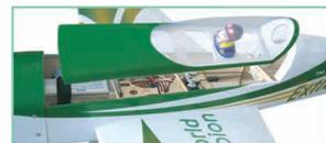
Detachable cockpit for easy access of battery compartment.
