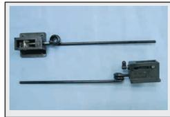
**Tail Gear with Spring shock Absorber (20-28 lbs)**
