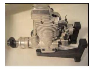
Drill the firewall for the motor mount using the blind nuts and machine screws in the hardware package to fasten the mount to the firewall.
