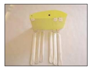
With a flat file or sandpaper, taper the edges of the cabane tabs so that the cabanes slide onto the tabs with ease.
