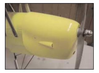
Mark and measure where your exhaust pipe or muffler will exit the cowl and make cutouts carefully. When satisfied with the fit, screw the cowl to the fuselage.
