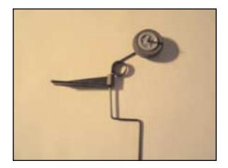
Using four 2x8mm screws, mount the tail wheel assembly to the rear of the fuselage, being careful to center the assembly.
