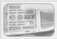
• Adjust the center position of the servo, then install it onto the servo mount by using screws and rubber blankets.
