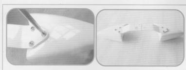
• Install the whell plant with 3 self-type screws(Just for Yak54 and SU26M/SU31).
