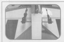
• Let the servo arm and rudder are at the center section, connect the cable and ball link as before.
