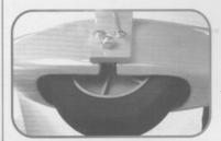
• If you assembly a Extra, you must install the axle first, and then install the wheel pant with two bolts. making sure the wheel is in the center of the wheel pant.
